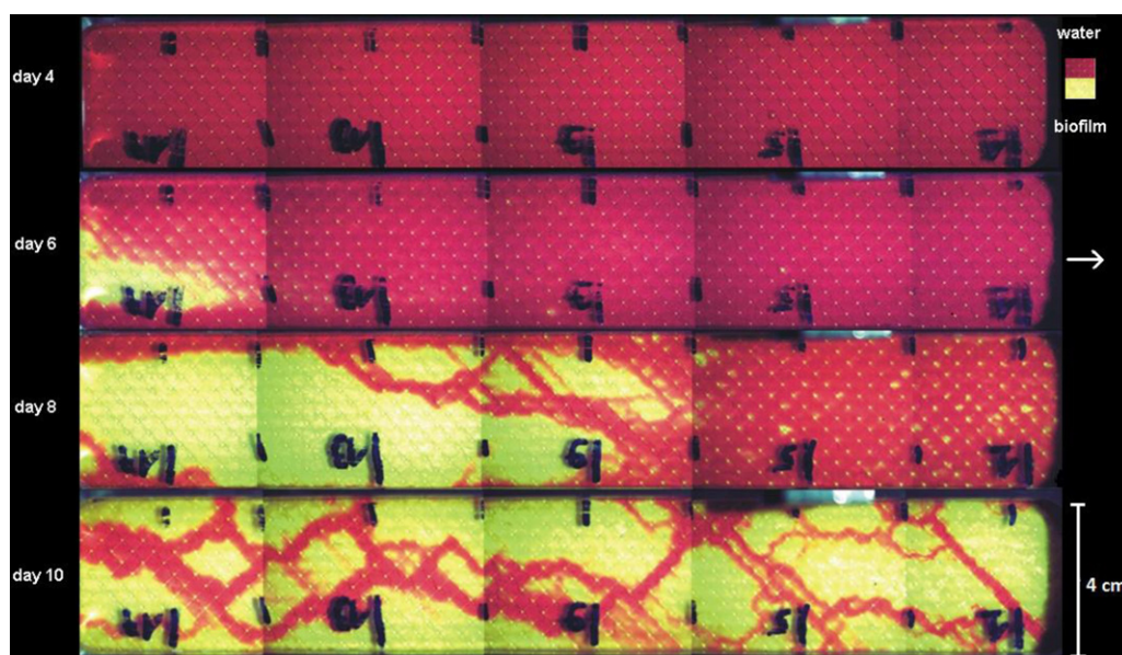
Fig. 6. Flow distribution in time due to biofilm development. A red dye (rhodamine WT) was dosed to the MFS feed water. Red coloured areas show regions of flowing water. Yellow coloured areas show stagnant water and biomass presence. Flow direction is from left to right (arrow). The width of the flow channel is 4 cm. (For interpretation of the references to colour in this figure legend, the reader is referred to the web version of the article.)
